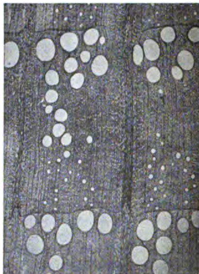
FIG. 2. — Cross-section of Ring-Porous Wood. (Red Oak.) (Bull. 126, U. S. For. Ser.)
